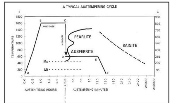
Fig. 2. A schematic representation of the CADI heat treatment cycle
