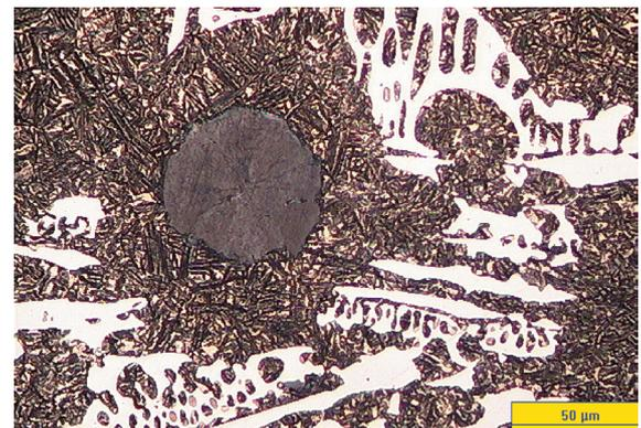
Fig. 3. A typical CADI microstructure showing carbide and spheroidal graphite, dispersed in an ausferrite matrix and austempered at 370°C
