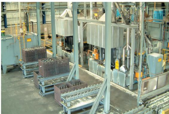
Fig. 1a. Purpose built furnaces for production of ADI and CADI. This facility at ADI Treatments Ltd operates the largest furnace of its kind in commercial use, accommodating parts up to 1.8m diameter
