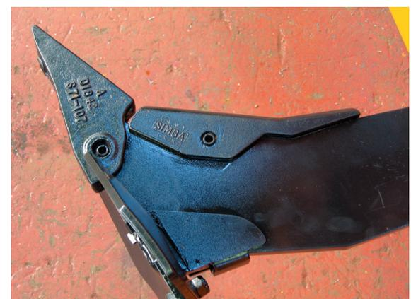
Fig. 4. Ground engaging components on the SIMBA Solo subsoiler. The CADI shank bearing the company logo is appositely positioned behind the white iron tip. Courtesy SIMBA International, www.simba.co.uk
